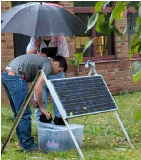
The seismograph stations installed at Ithaca High School to record the vibroseis waves as well as distance earthquakes to quantify ground response in Ithaca Valley. Professor Larry Brown observes May's work while holding an umbrella to protect them from the elements.
