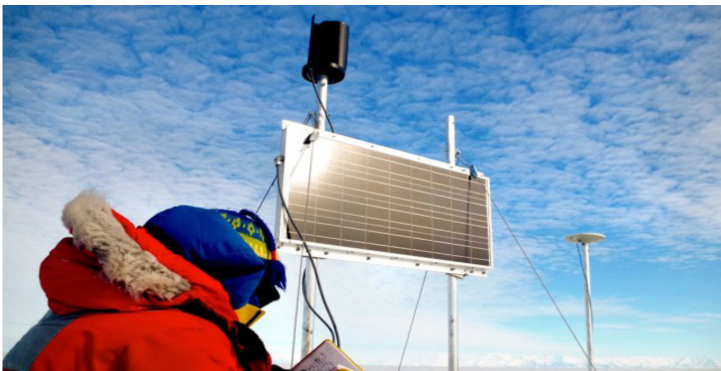
Matthew Siegfried inspects a GPS device, powered by a solar panel at Whillans Ice Plain.
