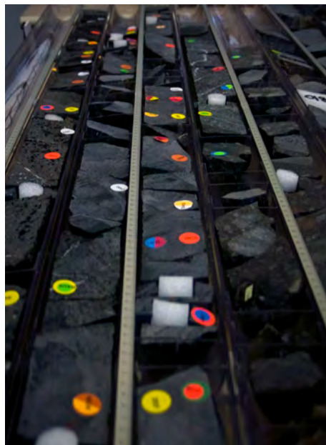
Core samples collected from a scientific drilling project, similar to samples that will be collected from the borehole. (Photo provided by Patrick Fulton)
